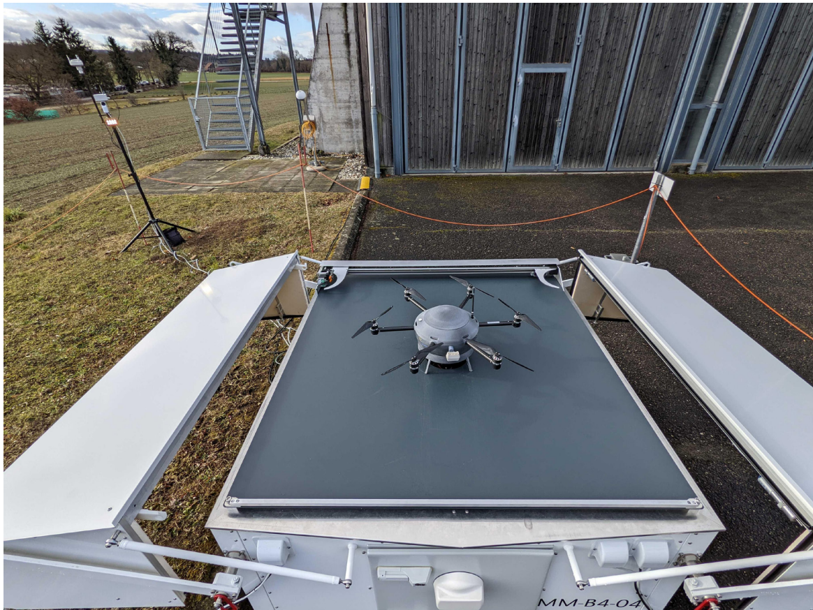
Figure 4. Meteomatics MeteoDrone MM-670 automatically recharging on the Meteobase
